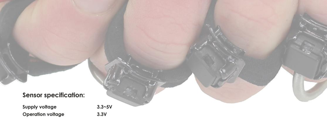
**Current consumption** 18mA Accelerometer range +/- 8g
